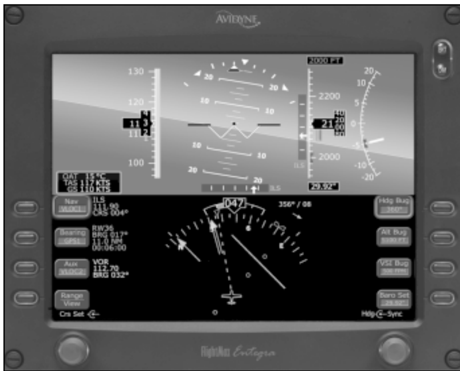
Above: Avidyne's FlightMax Entegra Primary Flight Display (PFD) replaces the standard instrument six-pack with a more intuitive instrument scan.
